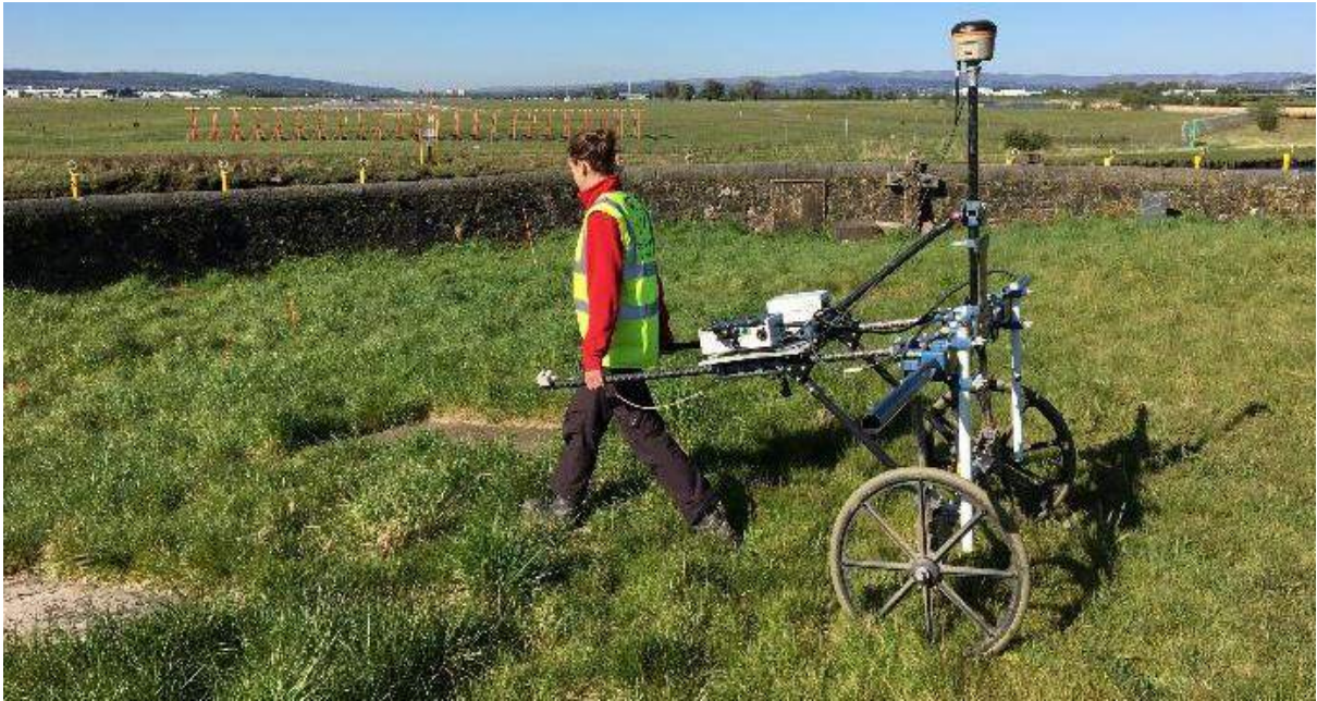
Magnetometry. The machine is measuring slight changes in the earth's magnetic field. Having the machine on wheels makes it a fast technique. © Calluna Archaeology.
