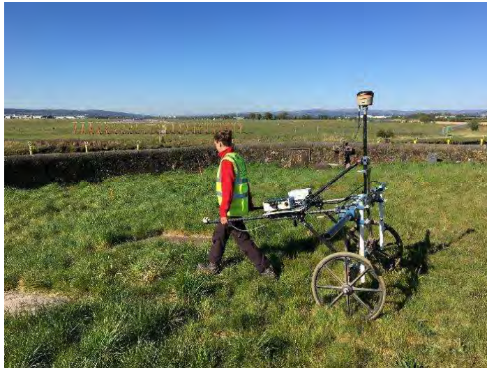
Magnetometry measures differences in the earth's magnetic field.
